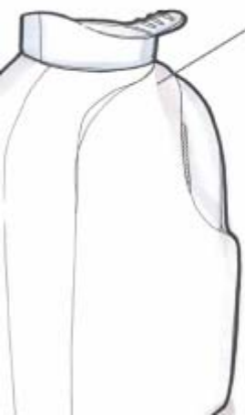
Material optimised handled bottle with minimal neck to reduce weight.
