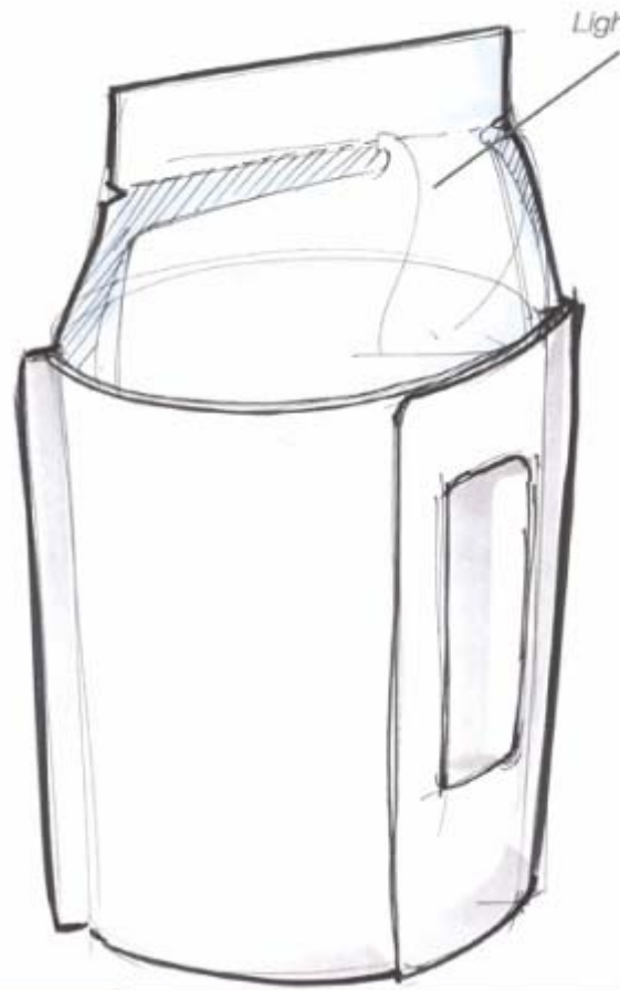
Material optimised handled bottle with minimal neck to reduce weight.
