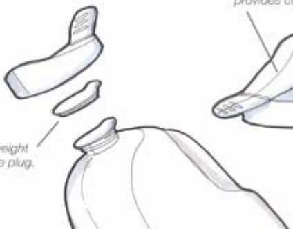
Screw on pouring spout provides control and re-close.
